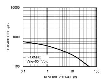
Fig.3 Typical Reverse Characteristics
